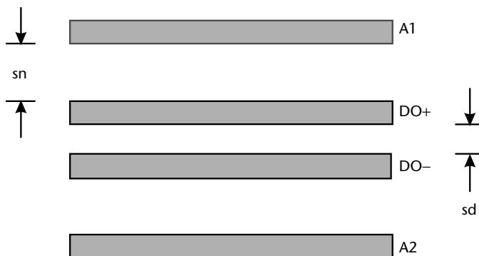
Figure 13.14 Top view showing four traces. Prevent common mode noise by making the spacing between the diff-pair ( sd ) smaller than the spacing to other traces ( sn ).
